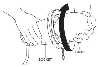
Figure 10. Installing the Lamp
